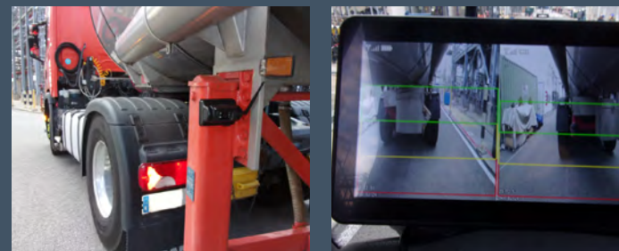
Proximity protection technology alerts drivers to the presence of pedestrians. Different types of technology are being implemented at Dow sites around the world.
